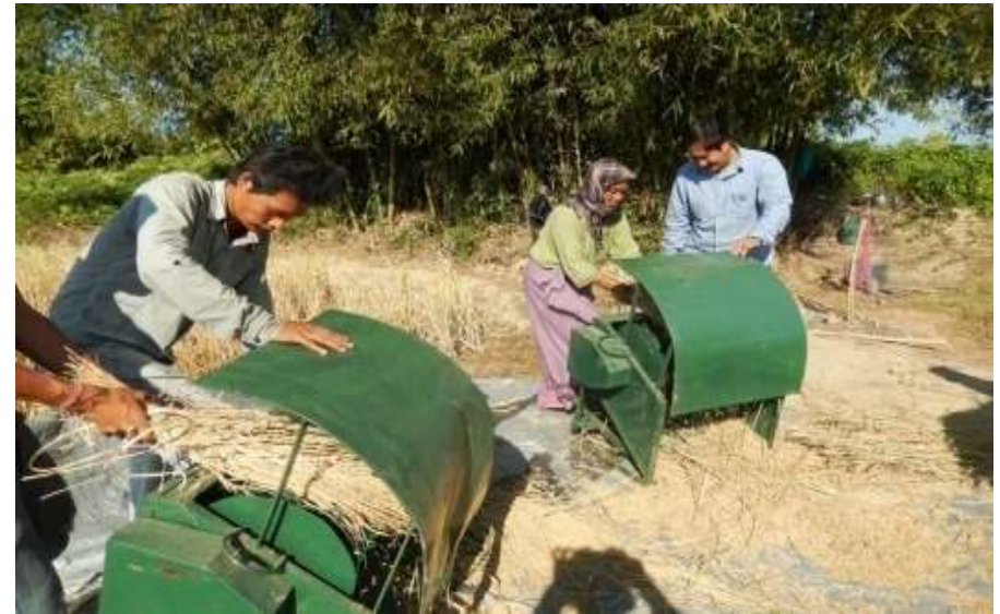
Threshing of paddy using Peddal Paddy Thresher at Runne Village
